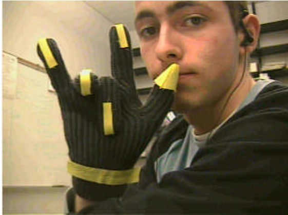
Fig. 1. Glove with six markers on the fingers, thumb and the wrist.
