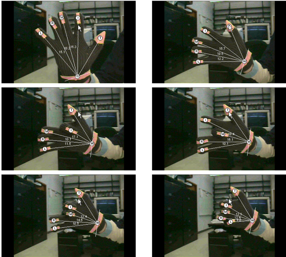
Fig. 4. Some results of the hand tracking. L (little finger), R (ring finger), M (middle finger), I (index finger), T (thumb) and W (wrist) label the features.
