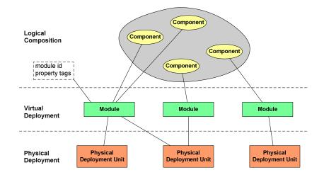
Fig. 5. Physical Deployment, Virtual Deployment and Logical Composition using Modules
